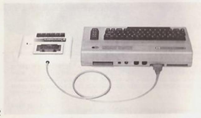
NOTE: When using the DATASSETTE™ with the Commodore 64, you should press the Commodore key to activate the DATASSETTE™ unit.
